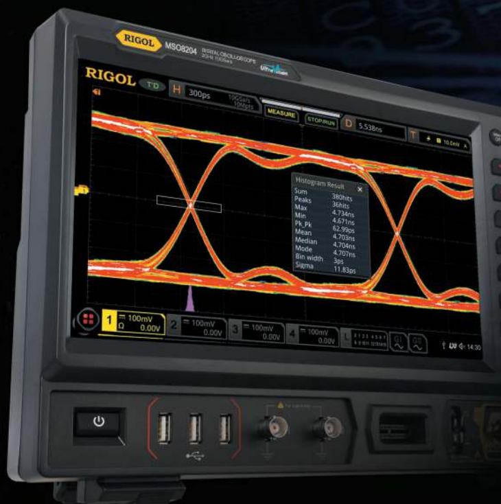
Perform eye measurement on the 622 Mb/s signal.
