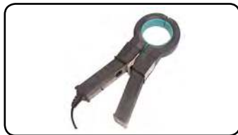
Current Clamp SC 2C 100A-1V
