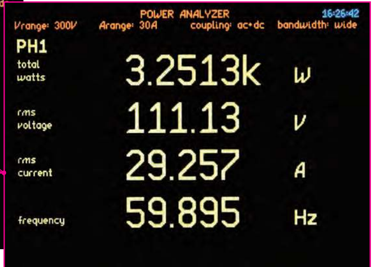
Zoom function enabled on total watts, rms voltage, rms current and frequency
