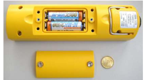
The battery compartment is opened easily using a coin. Two replaceable NiMH rechargeable batteries (AA size) are used to power the device.
