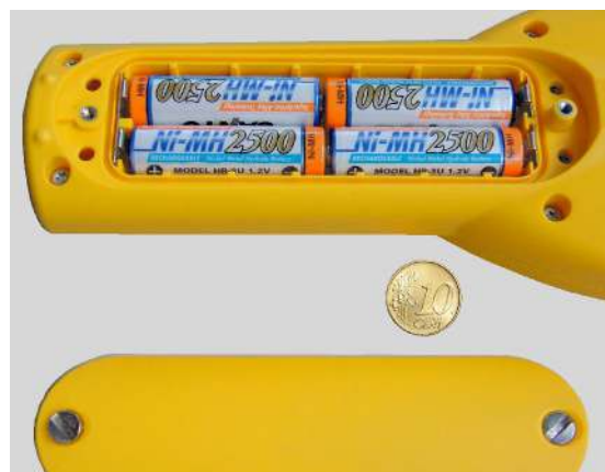
Above: The battery compartment is opened easily using a coin. Four replaceable NiMH rechargeable batteries (AA size) are used to power the device.
